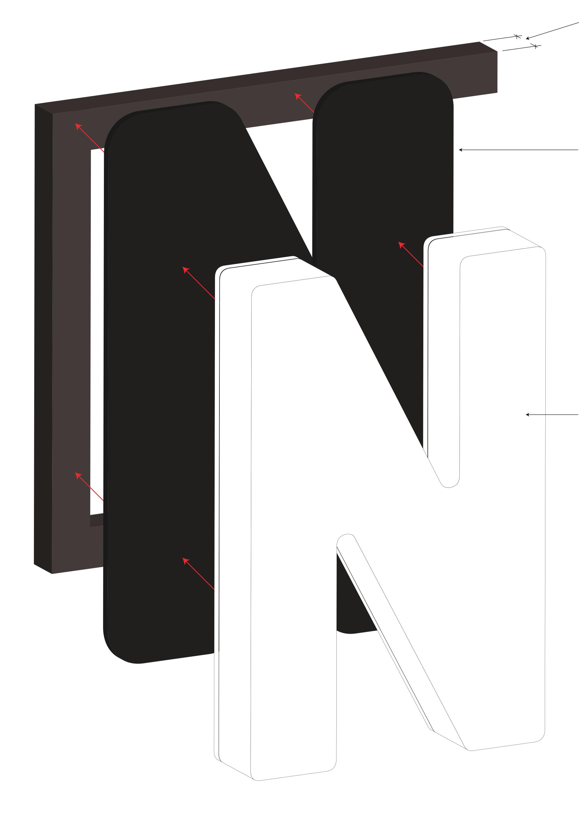
2" Fabricated/Welded Square Aluminum Tube Framing Painted To Match Existing Duranodic Storefront
